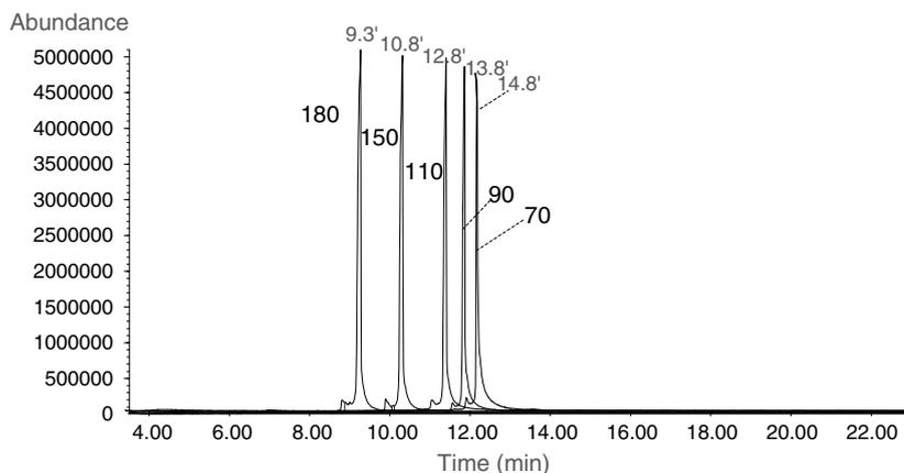
Fig. 2. Establishment of GC conditions for gestrinone. Each of the superimposed runs was run through an oven ramping procedure that began at the labeled temperature, held 2 min, then increased at  $20\text{ }^{\circ}\text{C min}^{-1}$  to a final temperature of  $280\text{ }^{\circ}\text{C}$ . The small peak preceding the prominent gestrinone peak is a 282 m.w. contaminant and likely represents loss of the acetylene side chain
