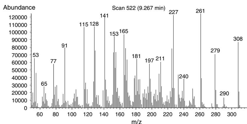
**Fig. 3.** Gestrinone EI-MS. Assignments:  $M^+$ , 308;  $m/z$  290, loss of water; 279, loss of  $CH_2CH_3$ ; 261 = 290 minus  $CH_2CH_3$ ; 227, partial loss of D ring [ $-C_6H_{10}$ ]; 211, loss of D ring [ $-C_7H_{13}$ ]; 197, loss of D ring [ $-C_7H_{12}O$ ]; 181, loss of B and D rings [ $-C_8H_{15}O$ ]; 91,  $C_7H_7$ ; 77,  $C_6H_5$ ; 65,  $C_5H_5$ ; 53,  $C_4H_5$
