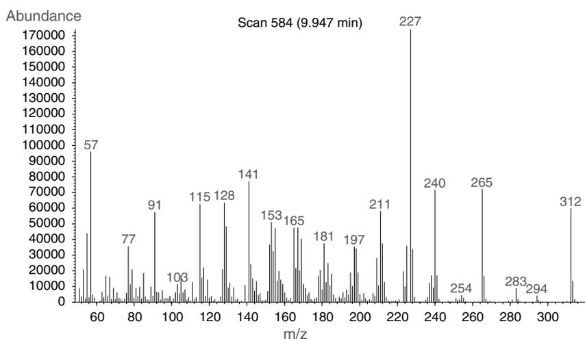
**Fig. 7.** Tetrahydrogestrinone final EI-mass spectrum. Notice that  $m/z$  values of only several high mass peaks changed significantly from those recorded for gestrinone (Fig. 3); gestrinone values listed in [brackets], including  $m/z$  312 [308], 294 [290], 283 [279], and 265 [261]. In addition,  $m/z$  233 was absent in contrast to gestrinone. The  $m/z$  values of the peaks in the remainder of the spectrum appear virtually identical to those of gestrinone
