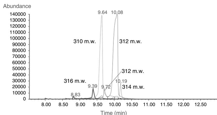
**Fig. 4.** Example of GC-MS of reaction products from a typical gestrinone hydrogenation experiment: Pd/SrCO<sub>3</sub> exposed to hydrogen for 10 min. A 100  $\mu$ L aliquot of the reaction in toluene was dried, resuspended in 1 mL ethyl acetate, and 1  $\mu$ L injected for GC-MS by the THG180 method. Selected ion chromatography revealed no 308 m.w. starting material, but candidates for single (310), double (312), triple (314), and even quadruple (316) double bond hydrogenations
